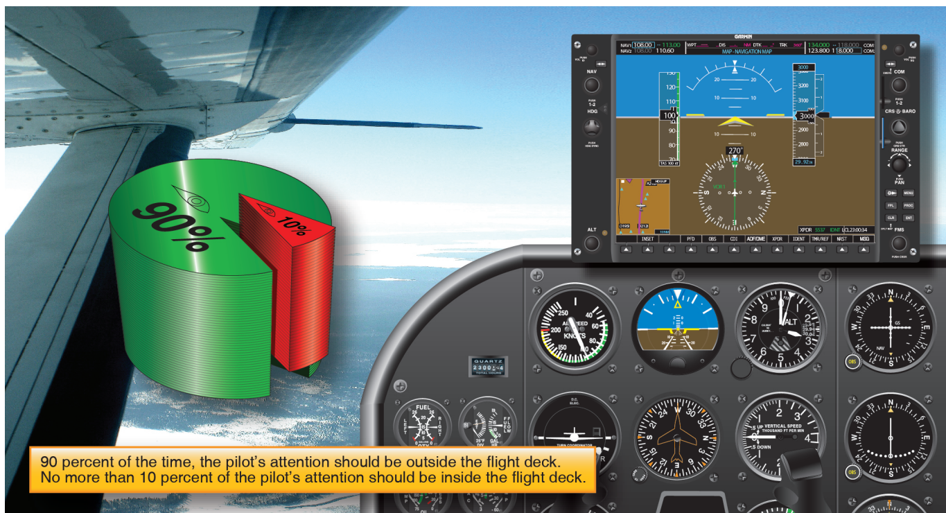
Figure 3-5. Integrated flight instruction teaches pilots to use both external and instrument attitude references.
