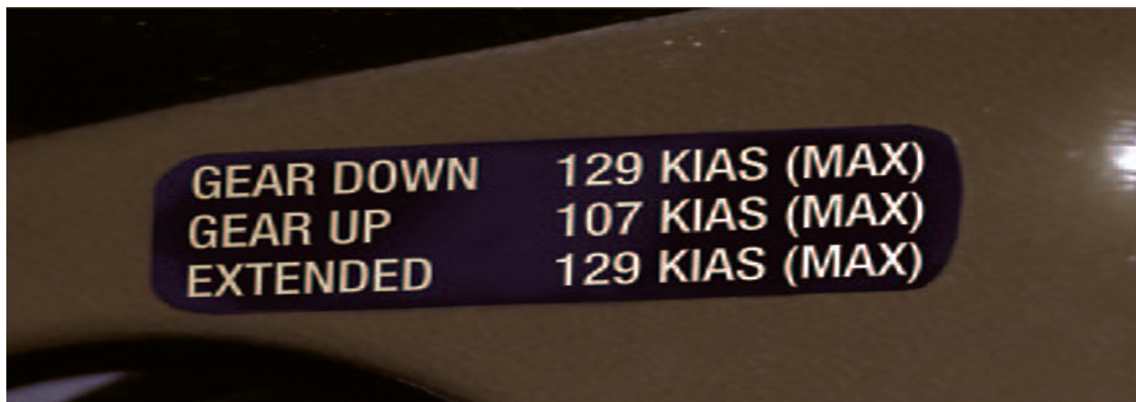
Figure 12-15. Placarded gear speeds in the flight deck.
